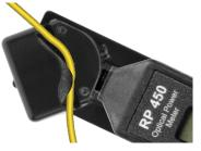
Insert fiber into LFI channel and pull trigger on unit to initiate macro bend in fiber. The LFI does not cause excess loss in the network.
