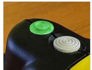
LED provides PASS/FAIL indication on the probe for fast verification of connector status.
